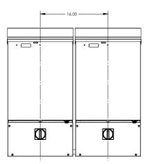
Example of Side-by-side Flush Mounting on 16" Intervals
